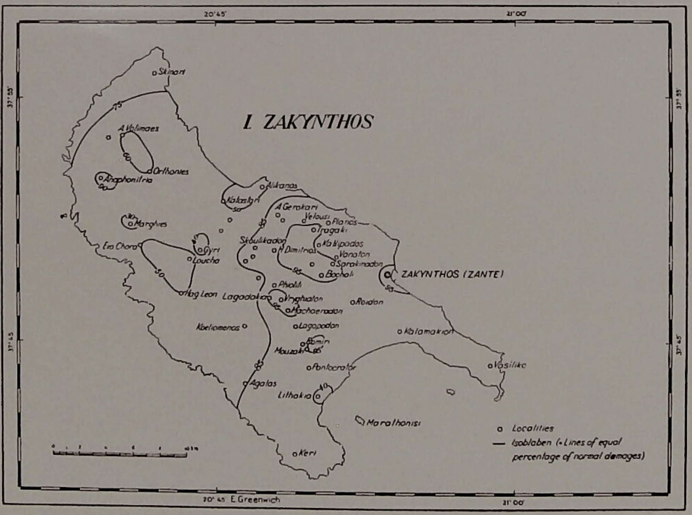
Fig. 3.—Distribution of the total damages on the Islands Cephalonia - Ithaca and Zante caused by the main earthquake of August 12, 1953, and its larger foreshocks and aftershocks.
