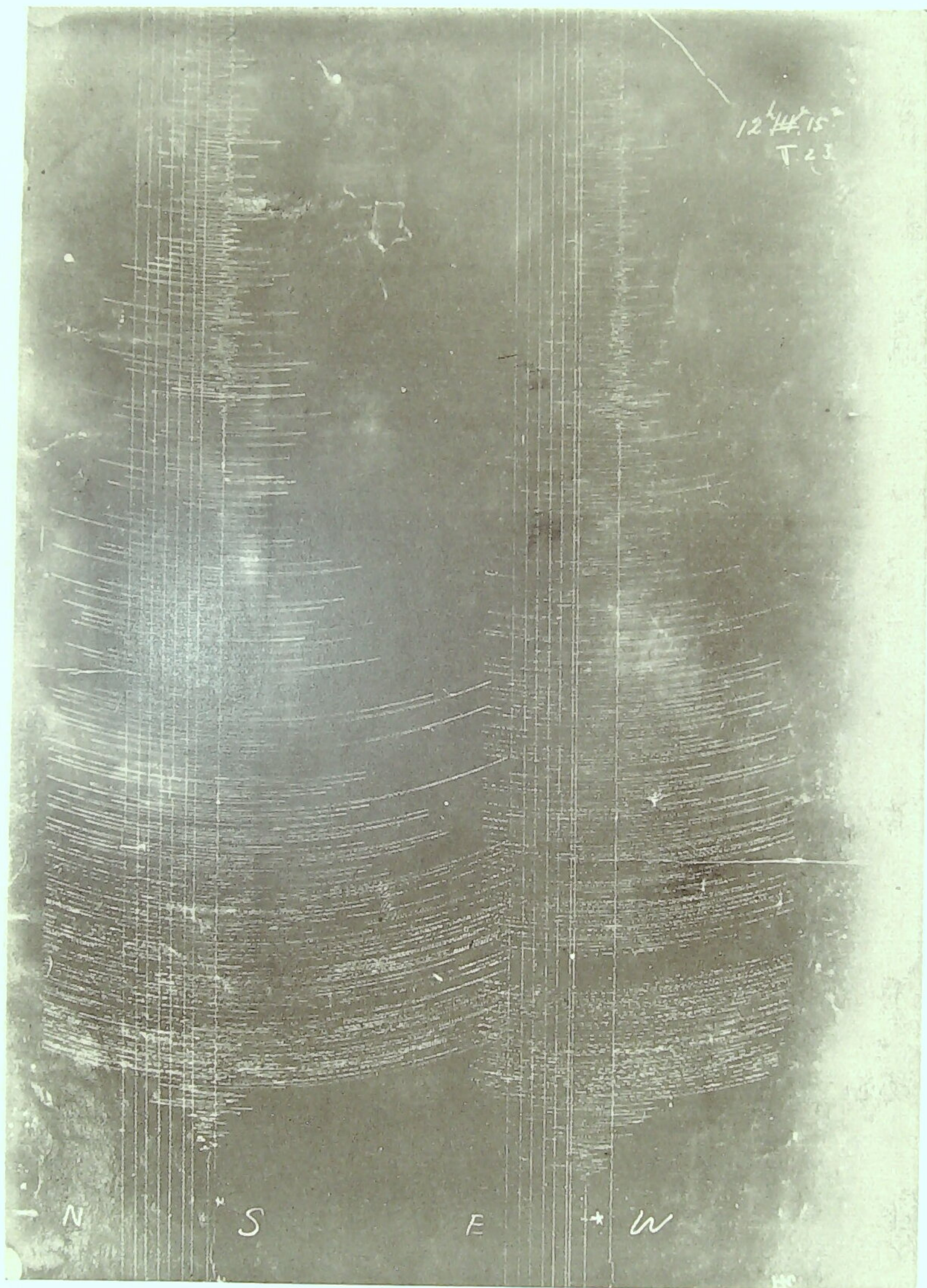
Tokyo Record of Wiechert's Horizontal Seismograph, North Tazima Earthquake occurred on May 23rd, 1925.
